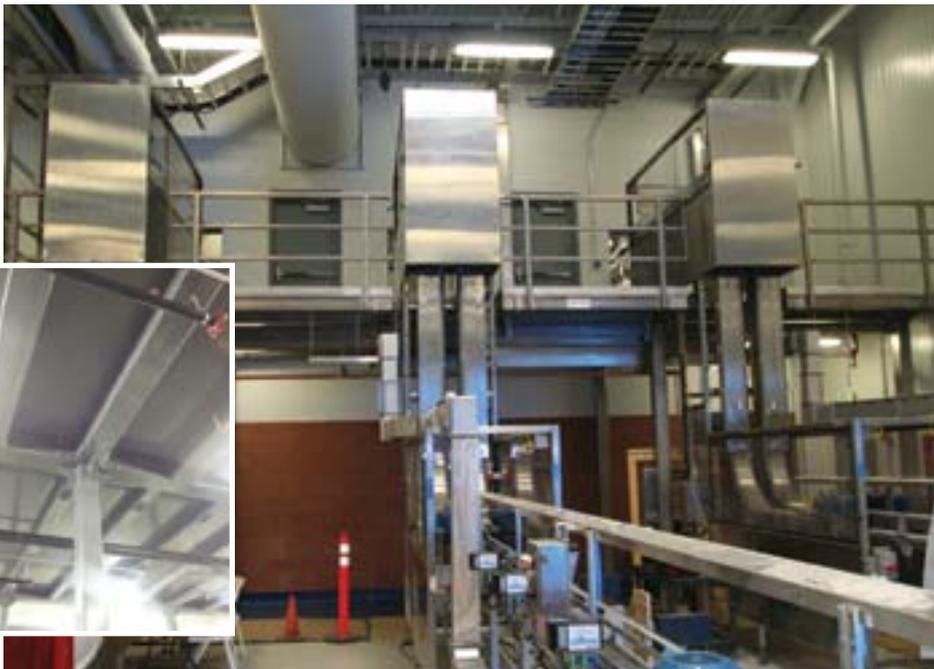
**Food grade platform used as a catwalk for multiple processing areas. Photo inset: All joints are designed to minimize cracks, crevices and protrusions and configured so as not to form traps, recesses or pockets.**
