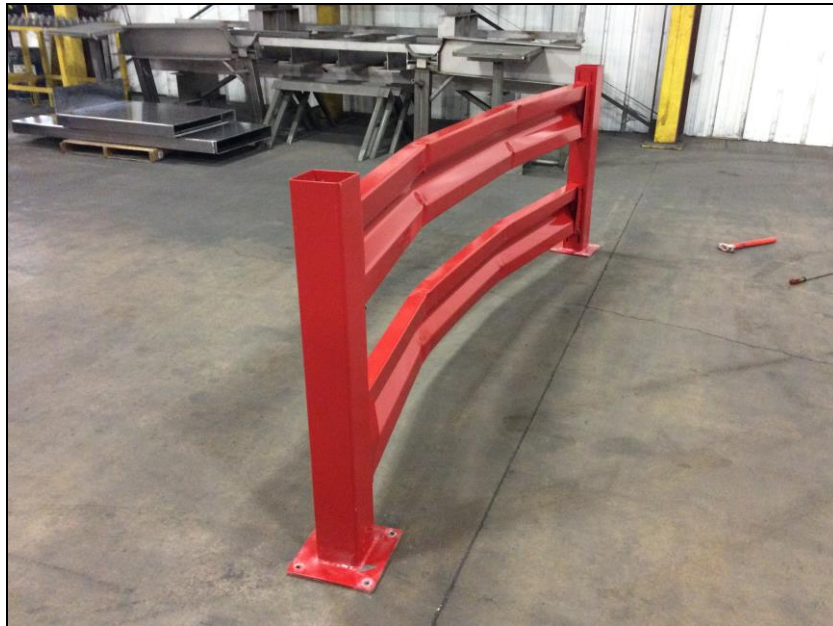
Photo 3: Deflection in the system after testing.
