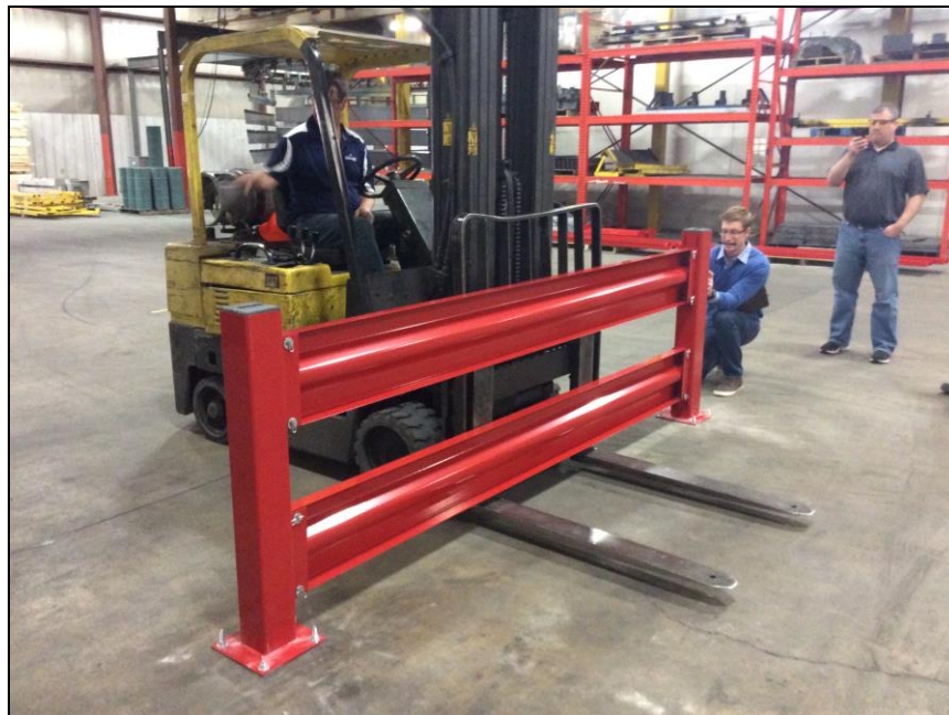
Photo 2: Alignment of the forklift with the system prior to testing.
